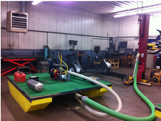
3” or 4” 23hp pump w/hookah air and nozzle
